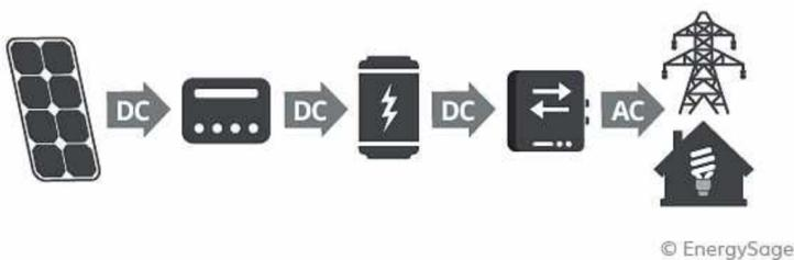
Example of DC-coupled system: DC electricity flows from solar panels to a charge controller and feeds it directly into a battery. An inverter is used to transform DC into appliance-friendly AC. Any electricity produced will be inverted once, flowing from your batteries to your home or out to the grid.
